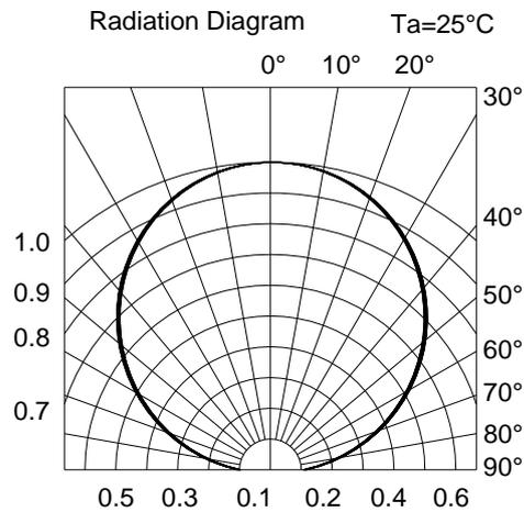
Typical Electro-Optical Characteristics Curves
